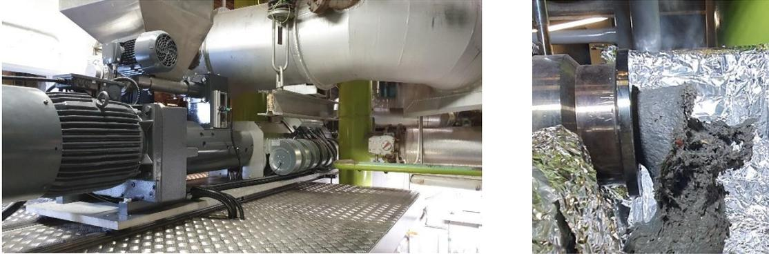
**Figure 4.** Feeding system via extruder used for this project in the left hand. Appearance of the melted material in the right hand.
